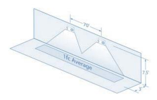
Using multiple DOE-HO units mounted at a typical 7.5' height delivers 63' on-center spacing with a 6' wide path of egress.
